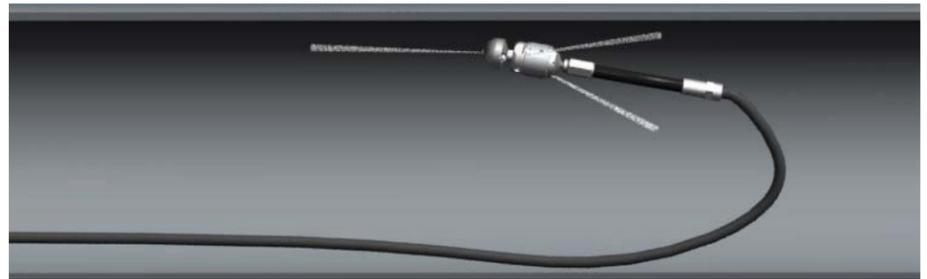
**Do not use the WS in 8 inch or larger pipe sizes, as the tool can turn around and come back toward the operator, causing serious injury or death.**
